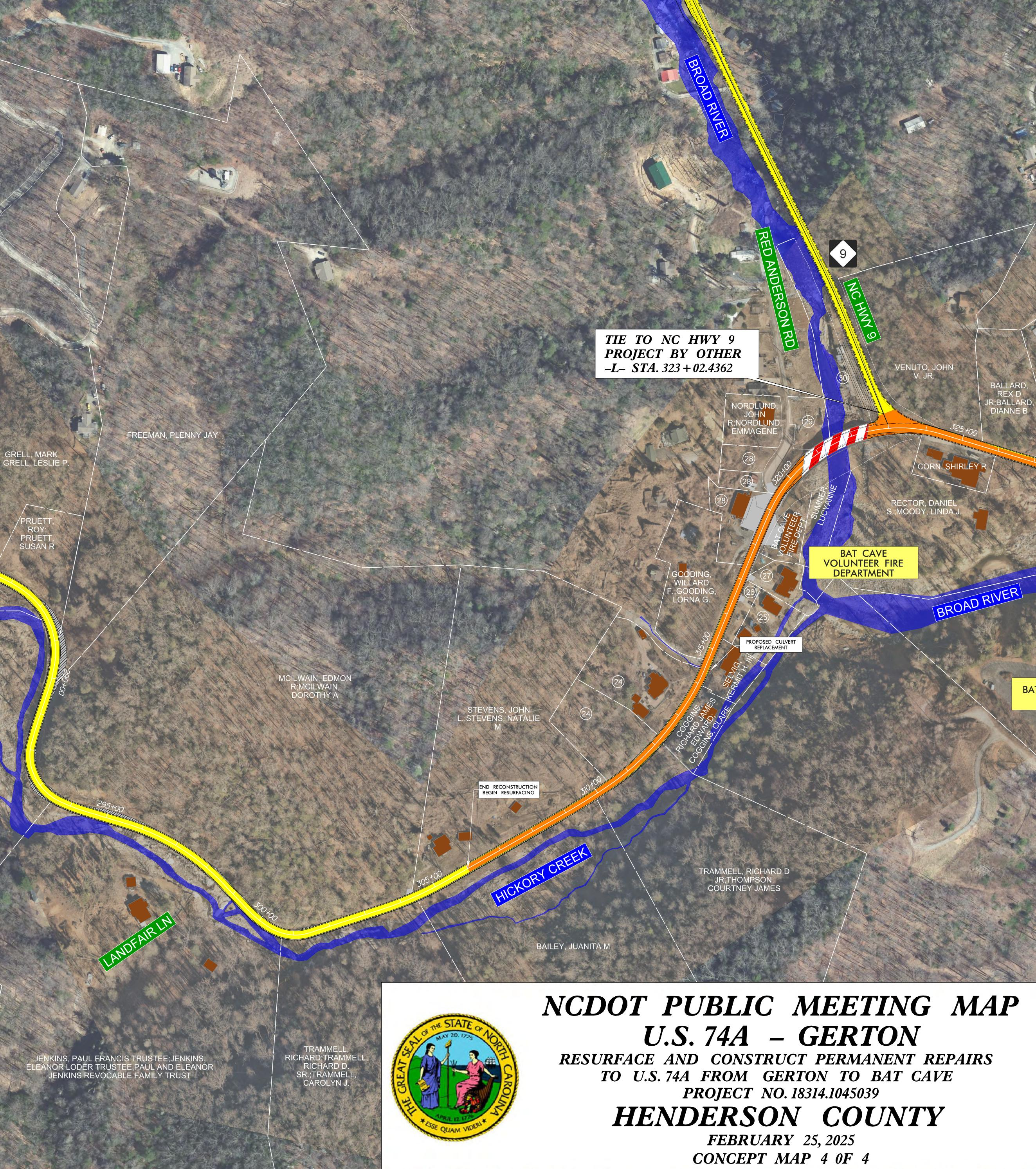
IMPACTS AND DRIVEWAY TIES: LIMITS OF CONSTRUCTION AND THEIR IMPACTS SHOWN ON THIS MEETING MAP ARE BASED ON PRELIMINARY DESIGNS AND GROUND SURVEYS. FINAL DRIVEWAY LOCATIONS WILL ALSO BE DETERMINED DURING FINAL DESIGN USING FINAL SURVEY.
