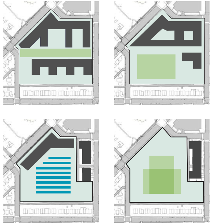
Various site plan scenarios for the future Western Bus garage block with residential development, a full-sized recreational field, and solar panels on the garage roof. These scenarios could involve a joint development partnership with neighboring properties on 44th and Jenifer Streets.
