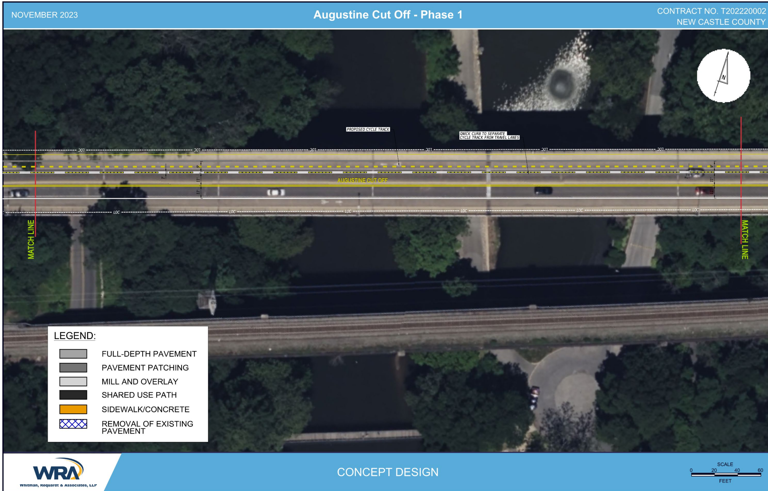
Figure 10. Proposed improvements, Augustine Cut Off Bridge
