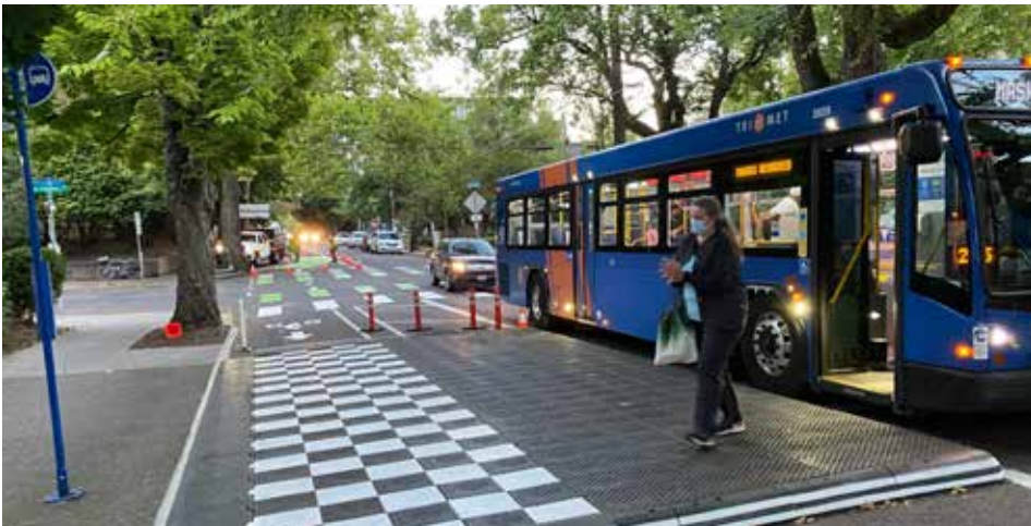
Figure 72. Level Boarding Platform with Protected Bicycle Facility
