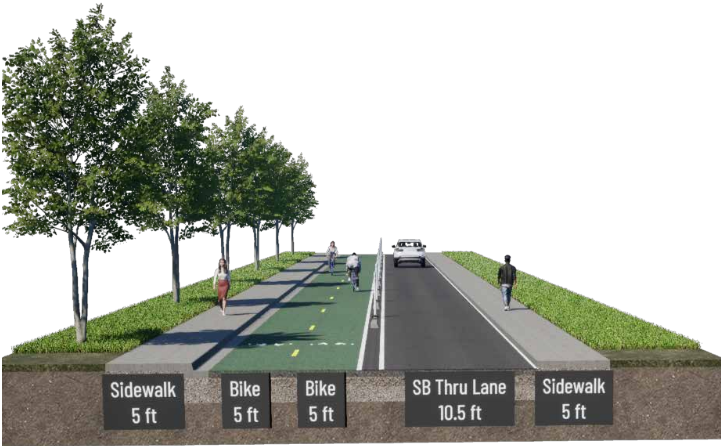
Figure 62. Concept for a Cycletrack on Adams Street from Rainbow Boulevard to 42nd Avenue
