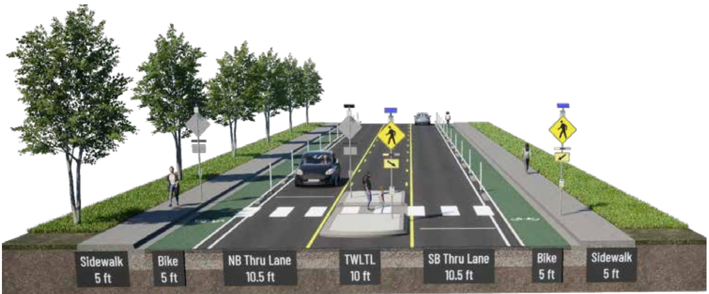
Figure 66. Proposed Pedestrian Crossing with Rectangular Rapid Flashing Beacon and Median Refuge Island
