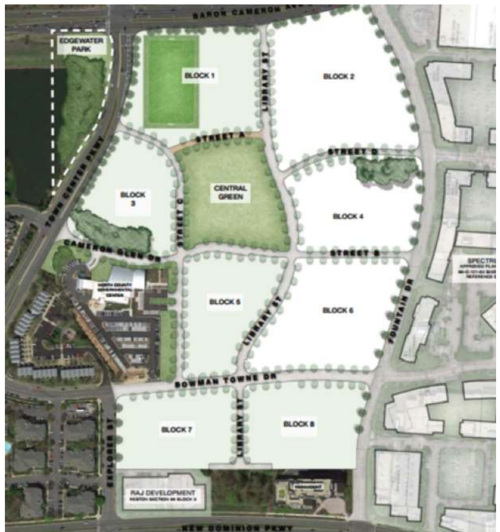
Below left: Concept diagram for the Public Open space at RTCN with the central green, rectangular field and grid of streets
