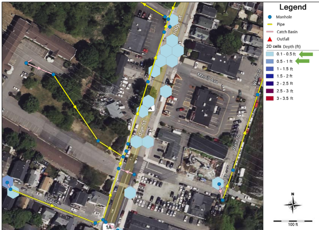
Figure 33: Bridge Street Model Predicted Flooding – 1 Year Rainfall – SCS Type III Distribution
