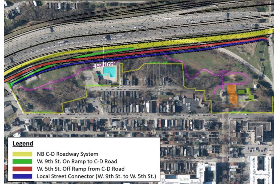
▲ Refined Alternative I (Concept I-W) | With extension of northbound frontage road between West 9 th Street and West 5 th Street (blue roadway).
