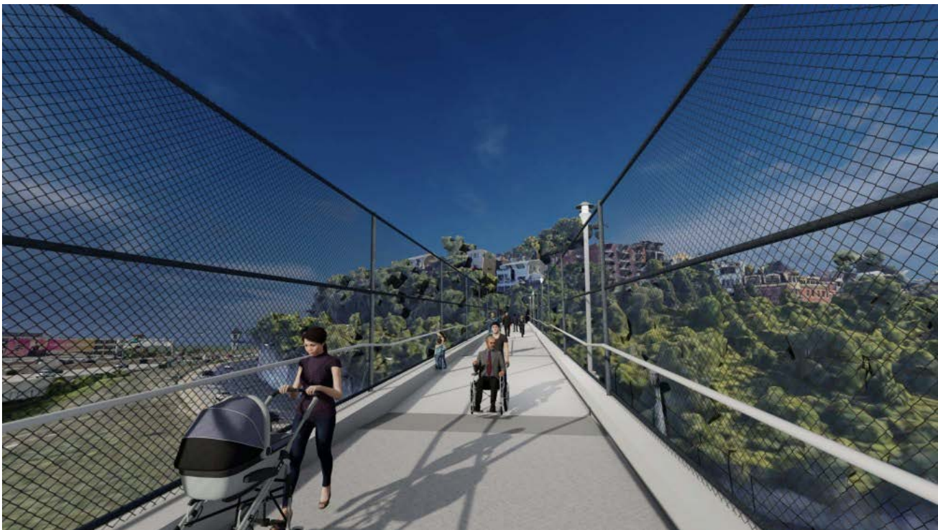
View of the Alternative 2 looking toward Mt. Adams. The darker areas on the bridge deck are flat respite areas that are five feet in length. (Click image to enlarge)
